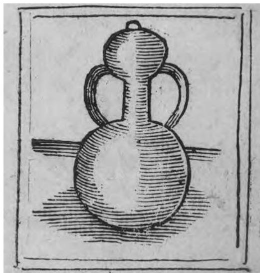
FIGURE 3. Pelican flask. “The matter must be put in at the top which afterwards Must be closed up.” From John French, *The Art of Distillation* (1651), title page (detail).
