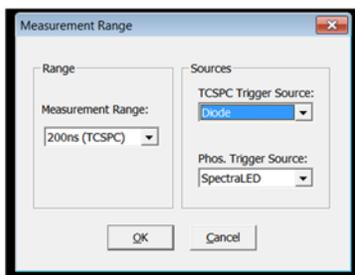
On the right hand side of the window, you will be asked about the Trigger source and Phos. Trigger Source. We currently have DeltaDiodes DD-330 and DD-280 for our DeltaFlex system, so the TCSPC trigger source should read “Diode.” Make sure to record which wavelength you are exciting the sample. (The value is written physically on the diode head). If you need to change excitation sources, contact Prof. Takematsu or Celeste for assistance.
