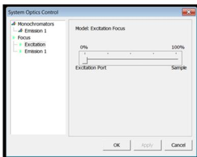
If you need to optimize the excitation and emission optics to increase your signal, you can either manually adjust each focal lens position by clicking on “Excitation Focus” and “Emission 1 Focus” under System Hardware and Optics, or you can go to Tools → Focus Scan and the program will automatically optimize the position of both focal lenses. The latter is recommended. Record the final positions of the lenses. You should always collect your sample decay and prompt under identical conditions.
