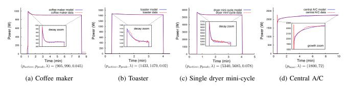
Fig. 7. An on-off growth/decay model closely matches the average power usage measured each second for a variety of resistive and inductive loads.
