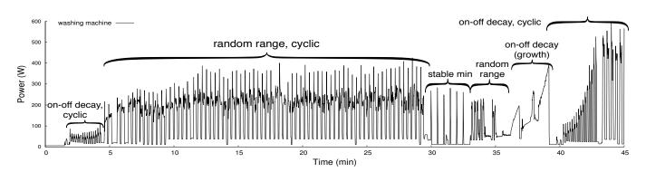
Fig. 10. A single complete cycle of a washing machinenannotated with the model types for the operation of simpler internal loads.
