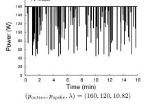
Fig. 9. A stable-max model of the LCD TV from Figure 1.
