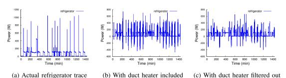
Fig. 15. Disaggregating refrigerator trace with the duct heater included and with the duct heater filtered out
