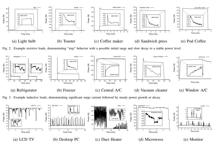
Fig. 4. Example non-linear loads, demonstrating rapid and significant random variations with possible ceilings and/or floors.
