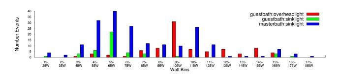
Fig. 7. Histogram of events for each 10W power bin for selected switches using the reactive learning technique.
