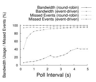
Fig. 11. Event-driven polling effectively utilizes bandwidth to monitor highly variable devices.
