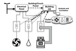
Fig. 1. Our monitoring and control architecture.
