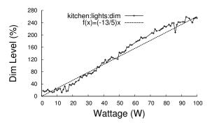
Fig. 6. Power usage is a linear function of a light's dim level.
