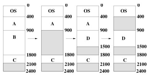
B terminates Allocate D A terminates
