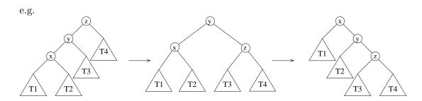
3. x has parent y and grandparent z and one of x and y is a left child and the other is a right child: rotate(x) followed by rotate(x)
