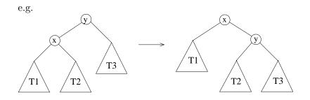
2. x has parent y and grandparent z and both x and y left (right) children: rotate(y) followed by rotate(x) Note: Does not work with rotate(x) and rotate(x)
