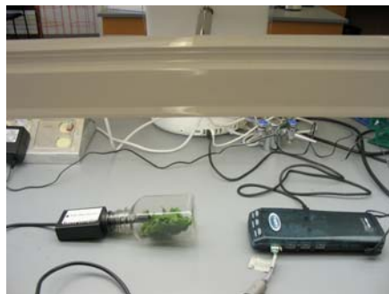
Figure 2. CO 2 sensor inserted in chamber containing spinach leaves
