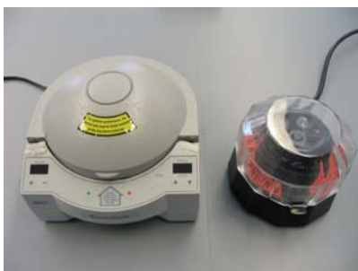
Figure 1. The types of microfuges available in the lab. The speed and spin time may be programmed into the centrifuge on the left. The centrifuge on the right has one speed and no timer.
