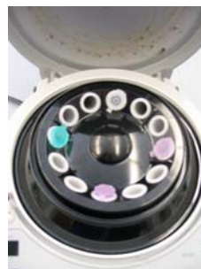
Figure 2. A balanced centrifuge. Always be sure there is a tube directly across from each tube and the tubes contain the same volume of liquid.
